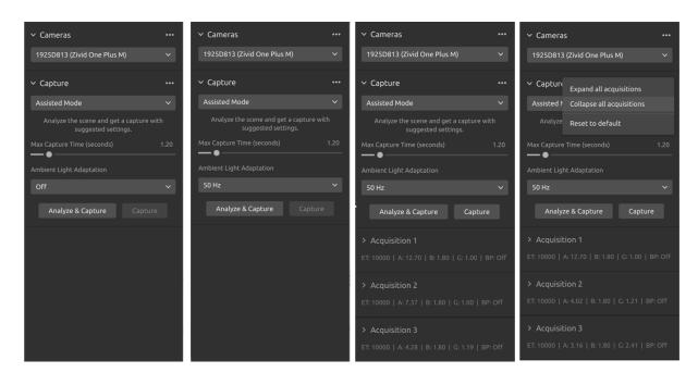
"Ambient Light Adaptation" is used when ambient light (AC powered) is mixed with the camera's projector.
