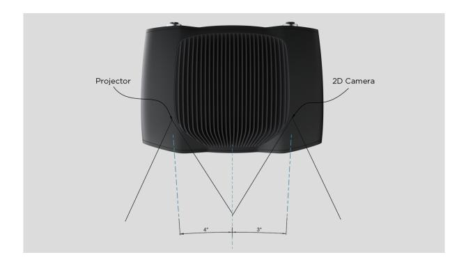
The 2D camera and the projector have an angle of 3 and 4 degrees with respect to the center axis. This should be considered if it is desired to have the camera perpendicular to the scene.
