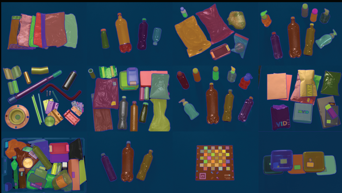
You can discover everything when you run the point clouds through a standard 2D-based AI segmentation algorithm.
