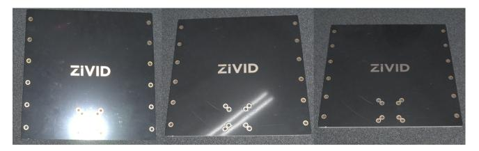
2D image with highlights from the projector (left), ambient light (center), and no highlights (right) depending on the camera position and angle.
