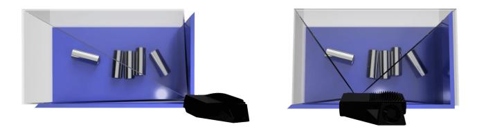
Mounting the camera this way minimizes interreflections from the bin walls, and also frees up space above the scene for easier access for tools and robots.
