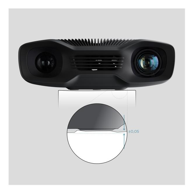
For optimal performance we recommend a mounting surface flatness of  $\pm 0,05$  mm or better. Mounting the camera to an uneven surface can in some cases affect the calibration.
