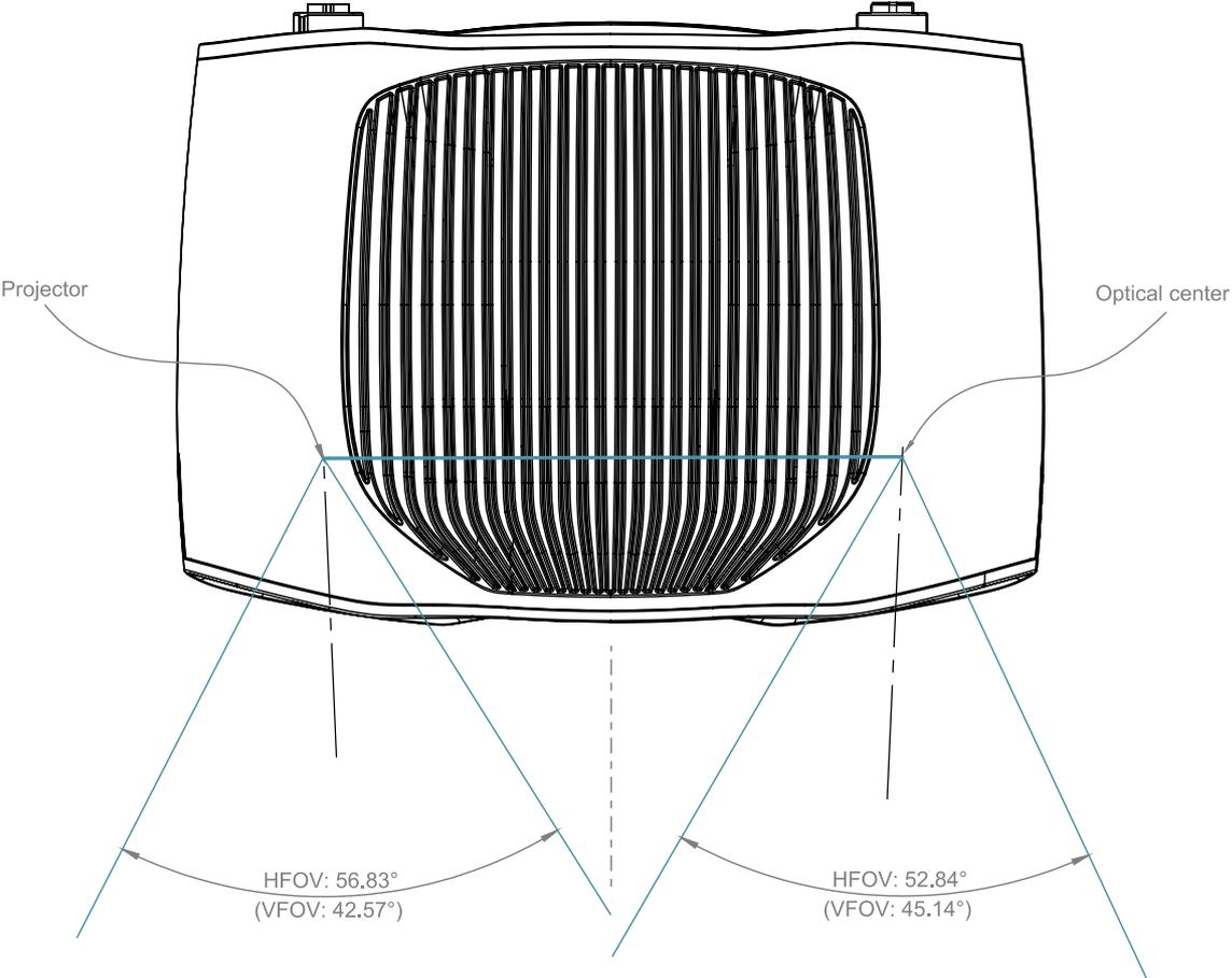
FIGURE 6 - OPTICAL CENTER POSITION RELATIVE TO MOUNTING HOLES
