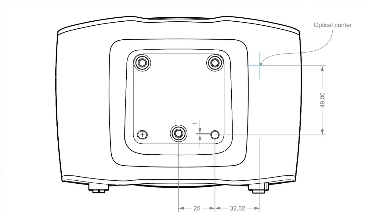
FIGURE 7 - OPTICAL CENTER POSITION RELATIVE TO BASE PLATE
