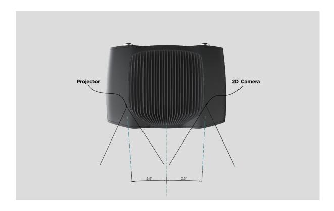
If possible, mount the camera at a slight tilt angle to avoid reflections and interference from the background. This also frees up space above the scene for easier access for tools and robots. With Zivid mounts it is straightforward to adjust camera mounting angles.
