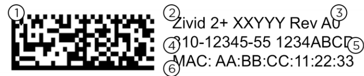
FIGURE 16 – UNIQUE ID LABEL EXPLANATION
