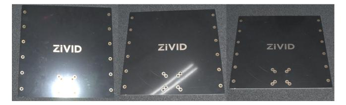
2D image with highlights from the projector (left), ambient light (center), and no highlights (right) depending on the camera position and angle.
