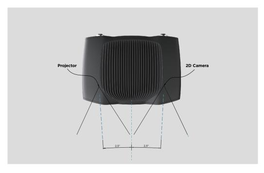
If possible, mount the camera at a slight tilt angle to avoid reflections and interference from the background. This also frees up space above the scene for easier access for tools and robots.
