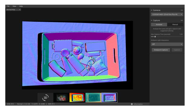
As a result, the normal map is useful for seeing planes in the point cloud. The normal map is also helpful in inspecting surface curvatures, surface textures, and transitions between objects.
