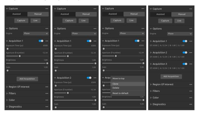
Once you select the manual mode, you can click the "Add Acquisition" button to add additional acquisitions. By default, each new acquisition added uses the settings of the previous acquisition. You can clone a specific acquisition by clicking on the three dots next to that acquisition and then on the "Clone" acquisition option. Use the same menu to reset acquisition settings or delete individual acquisitions. Disable or enable acquisitions with the checkbox.
