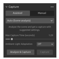
This triggers the camera to analyze the scene and output the camera settings required to cover as much of the dynamic range in the scene as possible. Immediately after this, the camera performs a second capture using these settings.
