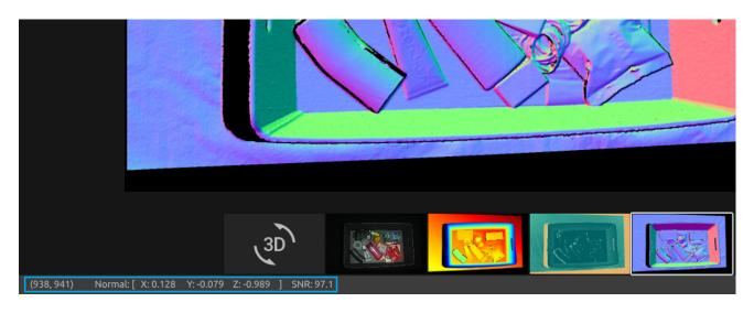
The normal map provides a 2D representation of the surface normals of a scene where RGB color components describe the normal vectors. For an introduction to normals, see the Normals Article .
