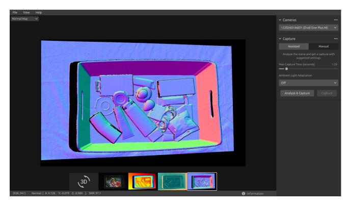
As a result, the normal map is useful for seeing planes in the point cloud. The normal map is also helpful in inspecting surface curvatures, surface textures, and transitions between objects as the color gradients describe these well.
