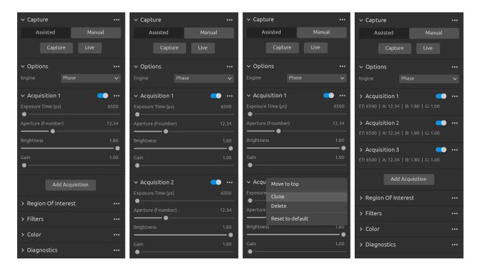
Once you select the manual mode, you can click the Add Acquisition button to add additional acquisitions. By default, each new acquisition added uses the settings of the previous acquisition. You can clone a specific acquisition by clicking on the three dots next to that acquisition and then on the Clone acquisition option. Use the same menu to reset acquisition settings or delete individual acquisitions. Disable or enable acquisitions with the checkbox.
