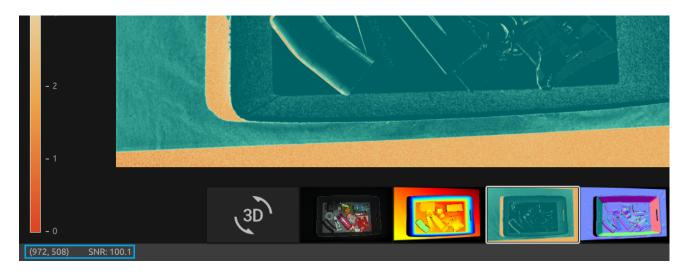
The color scale represents the variation in the SNR values. A pixel found at the higher end of the color scale represents a point associated with strong signal quality. For a point associated with a pixel found at the lower end of the color scale the ratio is more influenced by noise. Hence, these points involves higher uncertainty. For a detailed explanation, see the SNR values Article.
