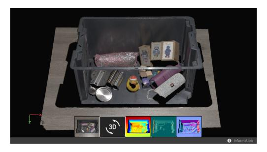
Turning color (C, D, R and S) and mesh (M) on and off in this view helps evaluate the point cloud quality.
