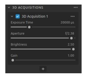
You can add multiple acquisitions within a capture by clicking the + button. This will allow you to capture the same scene with different exposure settings in an HDR capture, which can be useful for scenes with high dynamic range.
