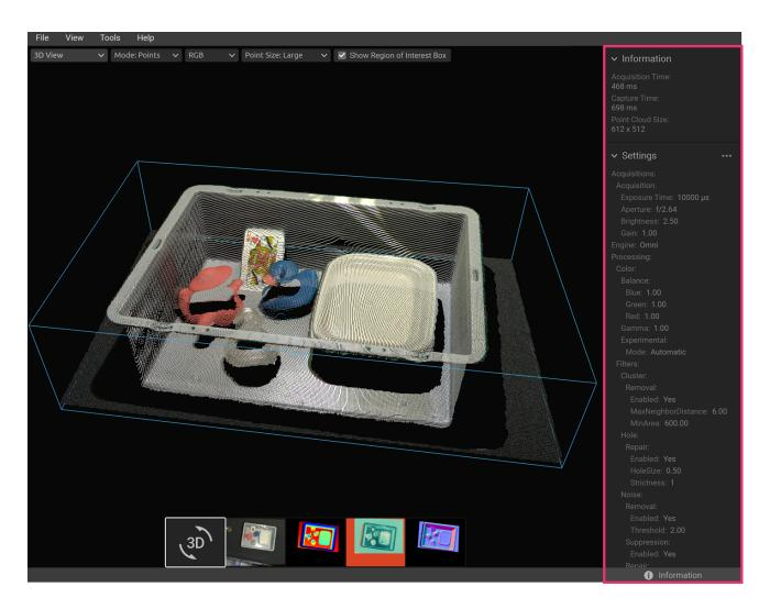
The bottom part shows the settings that were used in the capture. It is possible to save these settings to a file or apply them for use in the next capture.
