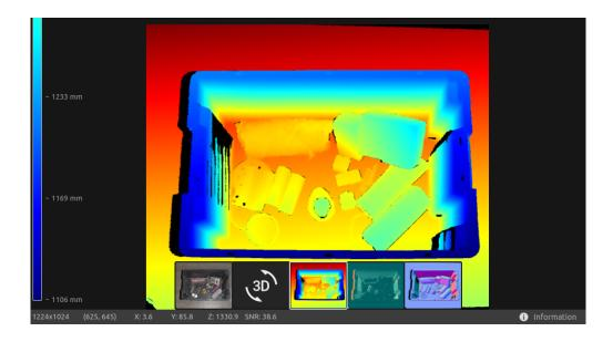
The color scale represents the distance variation along the z-axis from the camera to the surfaces of the imaged objects. To modify the range along the z-axis, you can use a fixed Z range in the top-left drop-down to narrow the color scale.
