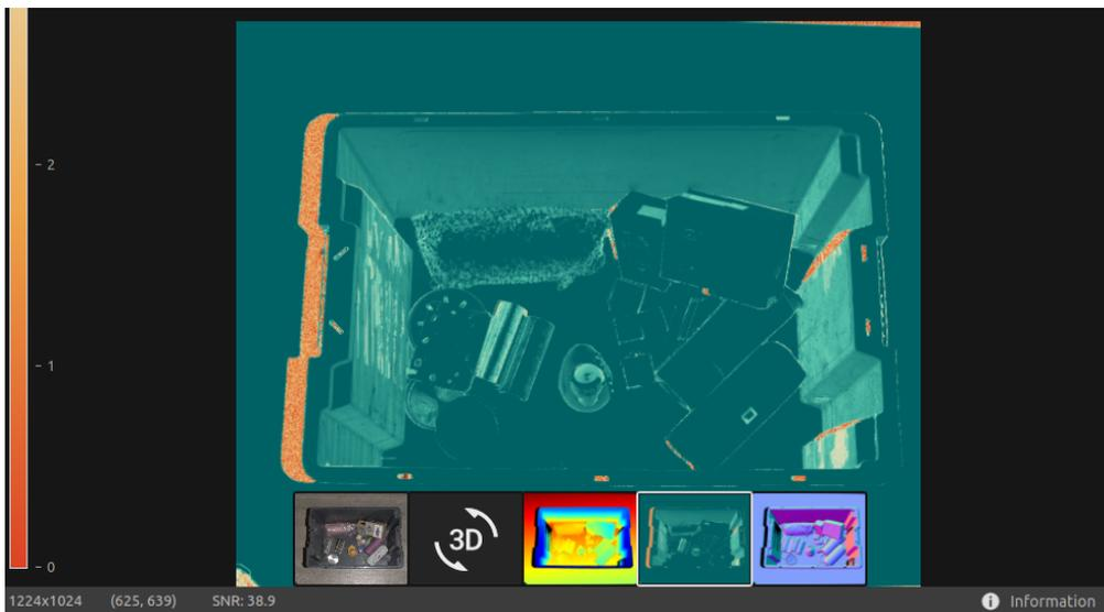
The color scale represents the variation in the **SNR values** . A pixel found at the higher end of the color scale represents a point associated with strong signal quality. For a point associated with a pixel found at the lower end of the color scale the ratio is more influenced by noise. Hence, these points involves higher uncertainty.
