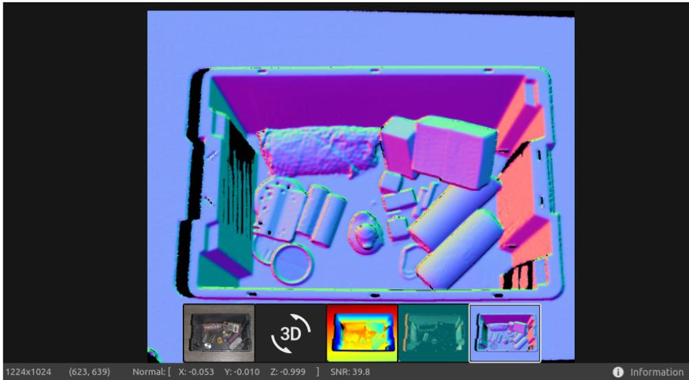
The normal map provides a 2D representation of the surface normals of a scene where RGB color components describe the normal vectors. It is helpful in inspecting surface curvatures, surface textures, and transitions between objects as the color gradients describe these well.
