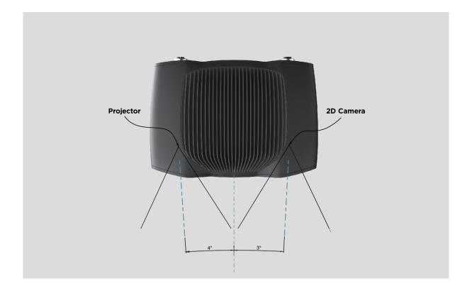
If possible, mount the camera at a slight tilt angle to avoid reflections and interference from the background. This also frees up space above the scene for easier access for tools and robots. With Zivid mounts it is straightforward to adjust camera mounting angles.
