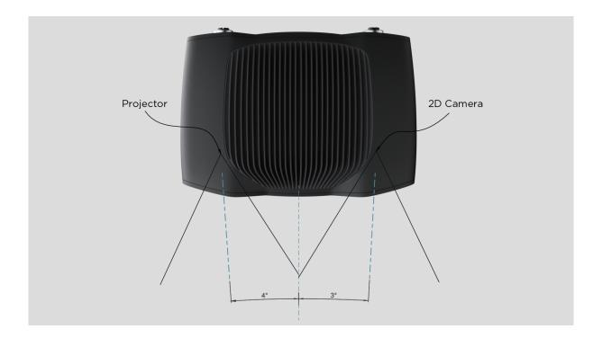
The 2D camera and the projector have an angle with respect to the center axis. This should be considered if it is desired to have the camera perpendicular to the scene.
