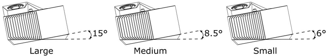
Although the most intuitive, this is not the best way to mount the camera. If possible, mount the camera at a slight tilt angle to avoid reflections from the background. This also frees up space above the scene for easier access for tools and robots.
